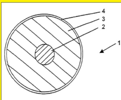
to the roller covering 3. The fluorinated rubber coating contains no filler or plasticizer and is approximately 25 µm thick. The outer surface of the fluorinated rubber elastomer coating 4 forms the outer surface of the roller, which is in contact with the damping solution or printing liquid.
